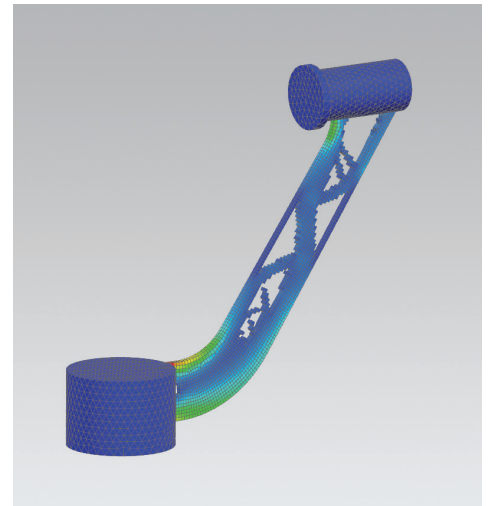
Optimized concept with stress results.
